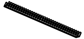
Edge Protector (1) (If the services hole is through a metal partition, the hole must be protected with the Edge Protector supplied to prevent damage to the power cord or hoses.)
